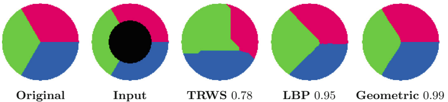
Fig. 4. Synthetic inpainting example. Here TRWS (truncated linear) shows the worst performance with only 78% correctly assigned labels. The values show ratio of correctly assigned labels and higher is better. LBP performs better than TRWS , but does not produce an interception of 120^\circ in the circle’s center. The update scheme of our geometric filter was terminated at entropy 10^{-4} , with a neighborhood 3 \times 3 and selectivity parameter \rho = 0.1 and produces the most accurate labeling.
