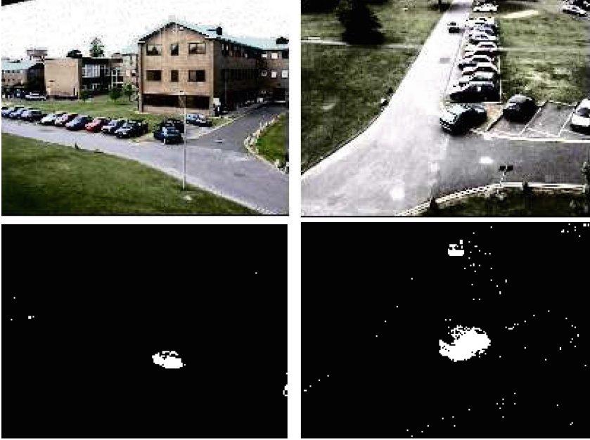
Fig. 3. Two camera views and their foreground masks obtained by background modeling
