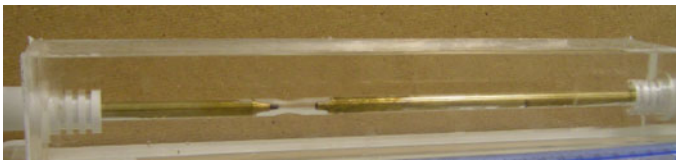
Fig. 12.4 Straight-tube stenosis phantom for use in PIV. The metal rods used in construction are shown positioned within the phantom
