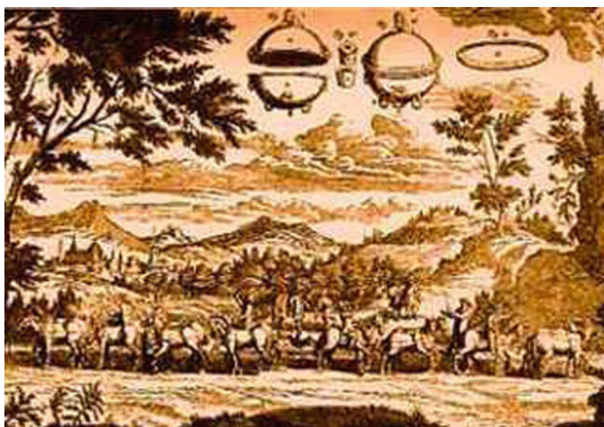
Fig. 1.11 Teams of horses trying unsuccessfully to pull apart vacuum-filled copper spheres in a Magdeburg demonstration for Emperor Ferdinand III. http://0.tqn.com/d/inventors/1/S/m/2/Magdeburg.jpg
