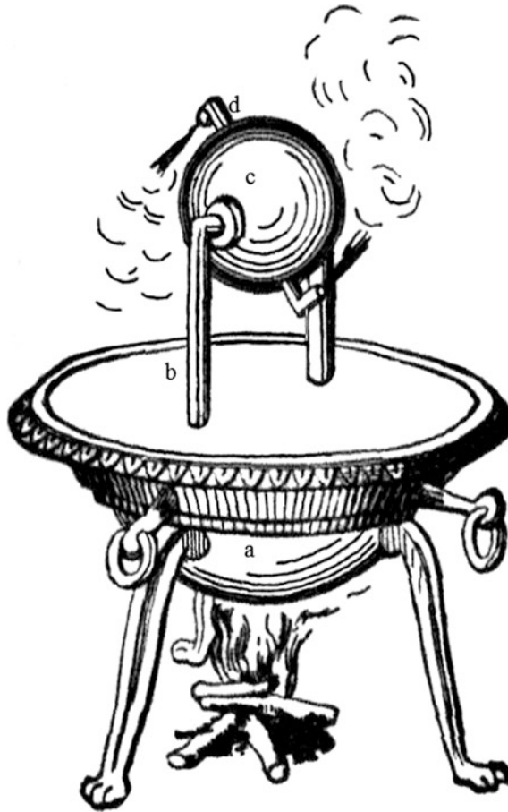
Fig. 1.4 Hero's aeolipile —the lower container “a” was partly filled with water and was heated. The steam that was then produced was led via pipes “b” to a metal sphere “c”, which could turn on its axle and had exhaust pipes “d”, whose openings were directed at right angles to the axle. As steam escaped, the sphere rotated because of the steam's reaction
