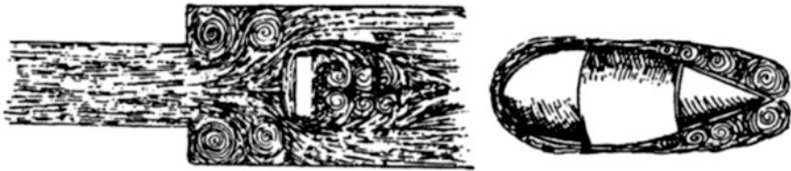
Fig. 1.10 Development of vortices in the separation region from Leonardo da Vinci. http://image.slidesharecdn.com/1-140906130430-phapp01/95/1history-5-638.jpg?cb=1410008998
