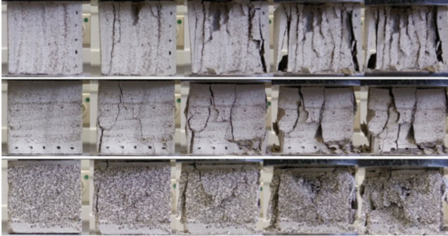
Fig. 7.19 Characteristic stages of the fracture behaviour for dry sprayed FGC cubes with an edge length of 100 mm tested parallel to the layers ( top ), dry sprayed FGC tested perpendicular to the layers ( middle ) and casted FGC ( bottom )
