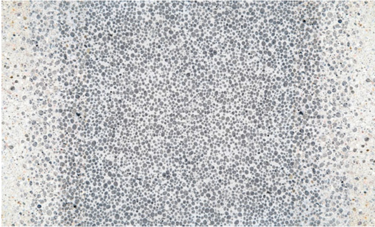
Fig. 7.16 Functionally graded exterior wall, U-value 0.275 \text{ W/m}^2 with wall thickness of 400 mm (Herrmann et al. 2013). The dark nodules consist of expanded porous glass
