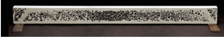
Fig. 7.15 Functionally graded concrete slab (100 mm thickness) with weight optimisation for load-bearing gravitational forces by using lightweight aggregates (Herrmann et al. 2013)
