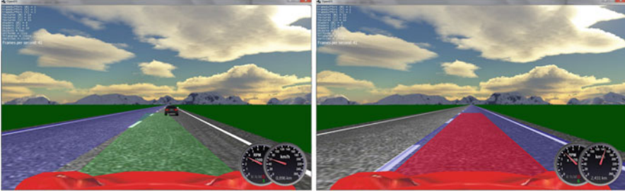
Fig. 4 Driver's view in OpenDS with integrated HMI for collision avoidance support. The system provides the driver with the visual representation of a proposed plan. The proposed lane to follow is highlighted by blue , the speed adjustment is proposed via green or red signal of appropriate intensity. There is an example of an instruction to change lane to left to overtake ( left image ). Second case shows how the red color informs the driver of proposal to slow down ( right image ) because of speeding in this case
