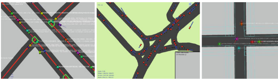
Fig. 2 Visualization layers in AgentDrive. The left image shows the graph visualization of the road network. Complex junction (city center of Prague) imported from OSM is in the middle image . The right image contains blue areas representing obstacle areas used by free-ride collision avoidance methods
