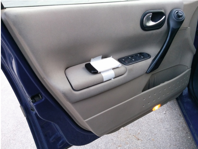
Fig. 2. Measuring of car door acceleration
