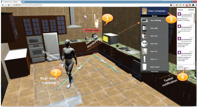
Fig. 7. 3D scene of the real-world on the Web browser. The microwave oven will be in a highlighted status (yellow) while it is being used; a steam is shown on the kettle icon when the real kettle in the kitchen is boiling water (circled 1), real-time location tracking (circled 2), visual service composition interface (circled 3) and social network notification in Twitter (circled 4). (Color figure online)
