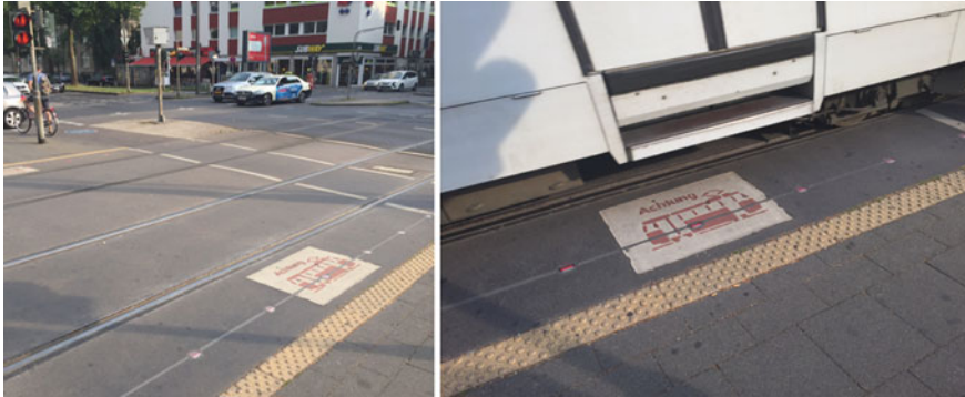
Fig. 21.3 New traffic lights anchored in the ground are tested in Cologne, Germany to prevent traffic accidents due to smartphone use (pictures by Christian Montag)
