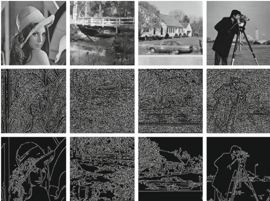
Fig. 3 row 1: Original images, Lenna, Bridge, House, Cameraman; Canny edge detected images at row 2: T = 0.005 , row 3: T = 0.2 for the \sigma = 0.5
