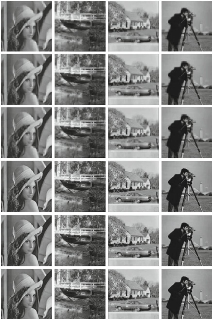
Fig. 4 Compressed images obtained using proposed algorithm (i) row 1 to row 3 for block size 16 \times 16 and thresholds (0.4 and 0.5), (0.3 and 0.4) and (0.2 and 0.35) respectively and (ii) row 4 to row 6 for block size 8 \times 8 and thresholds (0.4 and 0.5), (0.3 and 0.4) and (0.2 and 0.35) respectively for the test images of size 256 \times 256
