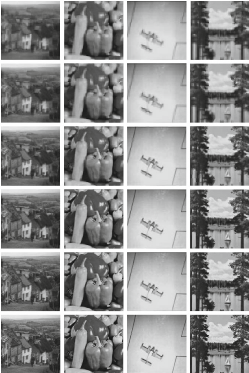
Fig. 5 Compressed images obtained using proposed algorithm (i) row 1 to row 3 for block size 16 \times 16 and thresholds (0.4 and 0.5), (0.3 and 0.4) and (0.2 and 0.35) respectively and (ii) row 4 to row 6 for block size 8 \times 8 and thresholds (0.4 and 0.5), (0.3 and 0.4) and (0.2 and 0.35) respectively for the test images of size 256 \times 256
