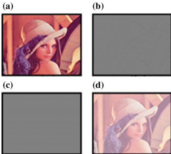
Fig. 4 a Color SI (FSDI), b Encrypted share1, c Encrypted share2, d Decrypted secret message
