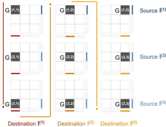
Fig. 2. M-Flash’s computation schedule for a graph with 3 intervals. Vertex intervals are represented by vertical (Source I) and horizontal (Destination I) vectors. Blocks are loaded into memory, and processed in a vertical zigzag manner, indicated by the sequence of red, orange and yellow arrows. This enables the reuse of input, as when going from G^{(3,1)} to G^{(3,2)} , M-Flash reuses source node interval I^{(3)} , which reduces data transfer from disk to memory. (Color figure online)
