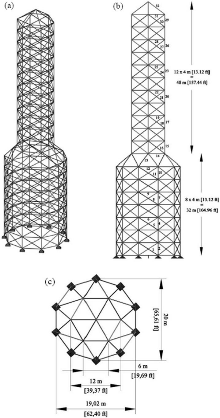
Fig. 7.17 Schematic of a 582-bar tower truss. (a) Three-dimensional view, (b) side view, (c) top view
