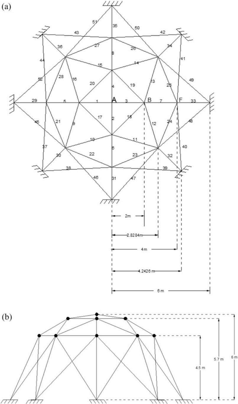
Fig. 7.20 Schematic of the 52-bar space truss. (a) Top view, (b) side view
