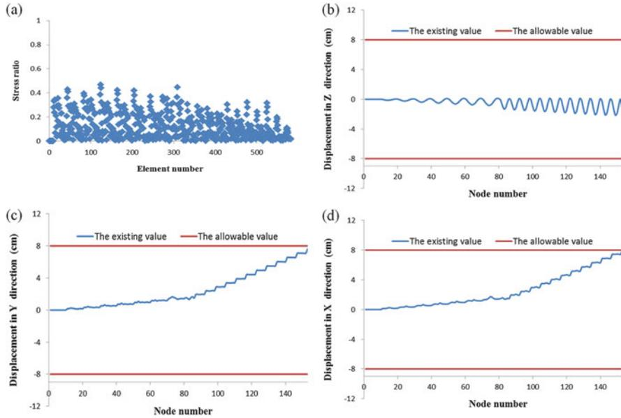
**Fig. 7.19** Comparison of the allowable and existing constraints for the 582-bar truss using the DHPSACO, [2], (a) stress ratio, (b) displacement in the z direction. (c) Displacement in the y direction. (d). Displacement in the x direction
