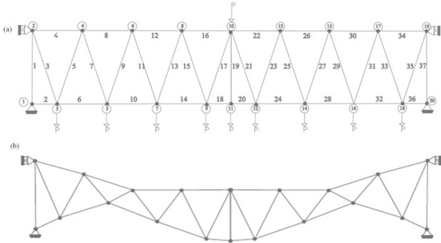
Fig. 7.9 (a) Schematic of the Forth Truss Bridge, (b) optimized layout of the Forth Bridge [2]
