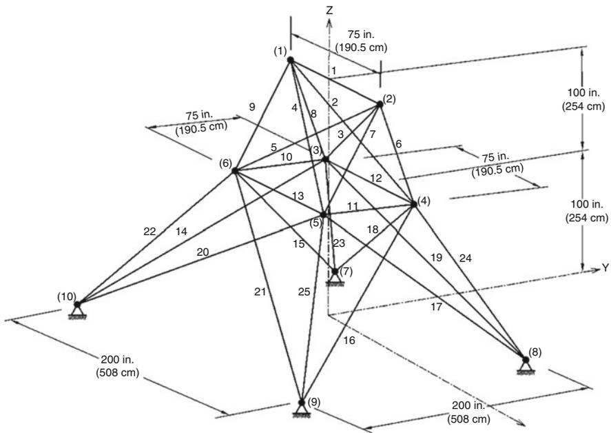
Fig. 7.12 Schematic of a 25-bar spatial truss
