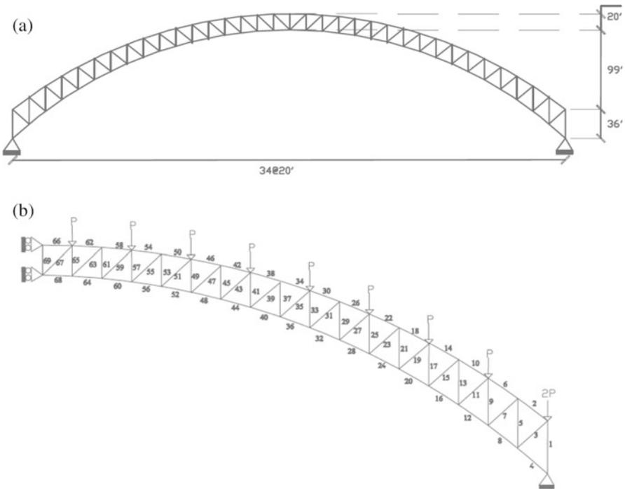
Fig. 7.22 (a) Schematic of the Burro Creek Bridge. (b) Finite element nodal and element numbering of Burro Creek Bridge
