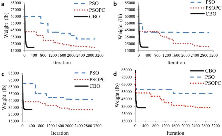
**Fig. 7.8** Convergence curves obtained for the different variants of the 120-bar dome problem [2]
