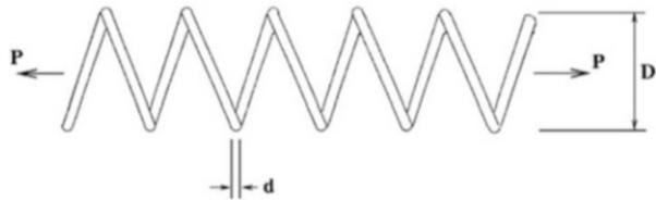
shear stress, surge frequency, and minimum deflection as shown in Fig. 7.6. The design variables are the wire diameter  $d (=x_1)$ , the mean coil diameter  $D (=x_2)$ , and the number of active coils  $N (=x_3)$ . The problem can be stated as follows:
