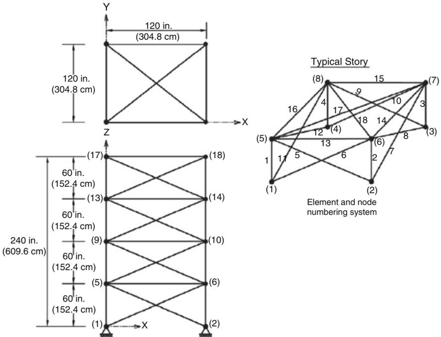
Fig. 7.14 Schematic of a 72-bar spatial truss
