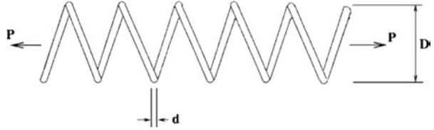
Fig. 14.3 Schematic of the tension/compression spring with indication of design variables
