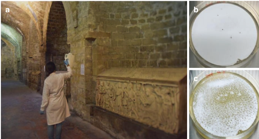
Fig. 2.3 Crypt environment. (a) Aerosol active sampling by portable sampler equipped with sterile disposable gelatin filter; (b) nutrient medium inoculated by gelatin filter (completely water-soluble); (c) dissolving of gelatin filter during the contact with Nutrient Agar (the filter completely disappears in 10 min)
