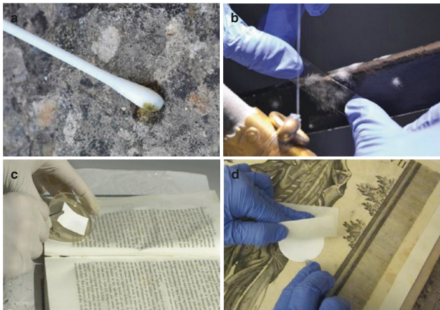
Fig. 1.4 Noninvasive sampling tools: (a) cotton swab on stone, (b) adhesive tape on lather, (c) nylon membrane fragment on book and (d) nitrocellulose membrane on paper (drawing)
