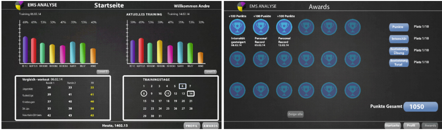
Fig. 12. The figure shows two exemplary screenshots of a gamified information application for users of electro muscle stimulation training [137]. The screen on the left shows stimulation intensities of different body parts in the last training session compared to a reference session and date picker UI components for selecting the respective sessions. The right screen shows a reward screen with a gallery of achievement badges and a total score. Augmenting trainer discussions with small interaction sessions with such performance-oriented applications was shown to lead to improvements in some motivational measures.
