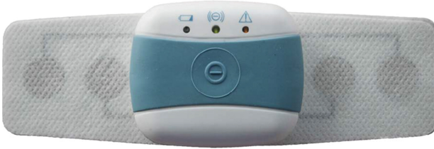
Fig. 1. Pulse Sensor. The two external electrodes inject the current, while those in the middle read the difference in electric potential. The Pulse Sensor can either analyze onboard, store or transmit the ECG tracings.
