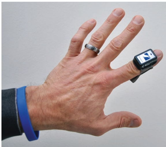
Fig. 10.5 The Kinesia One™ sensor, which is placed on the fingertip and can monitor motor symptoms of PD, image provided courtesy of Kinesia
