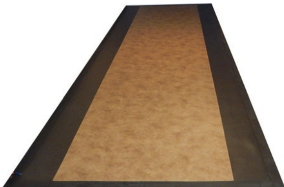
Fig. 10.2 The Zeno™ walkway carpet system used to monitor gait performance in real time, image provided courtesy of Protokinetics
