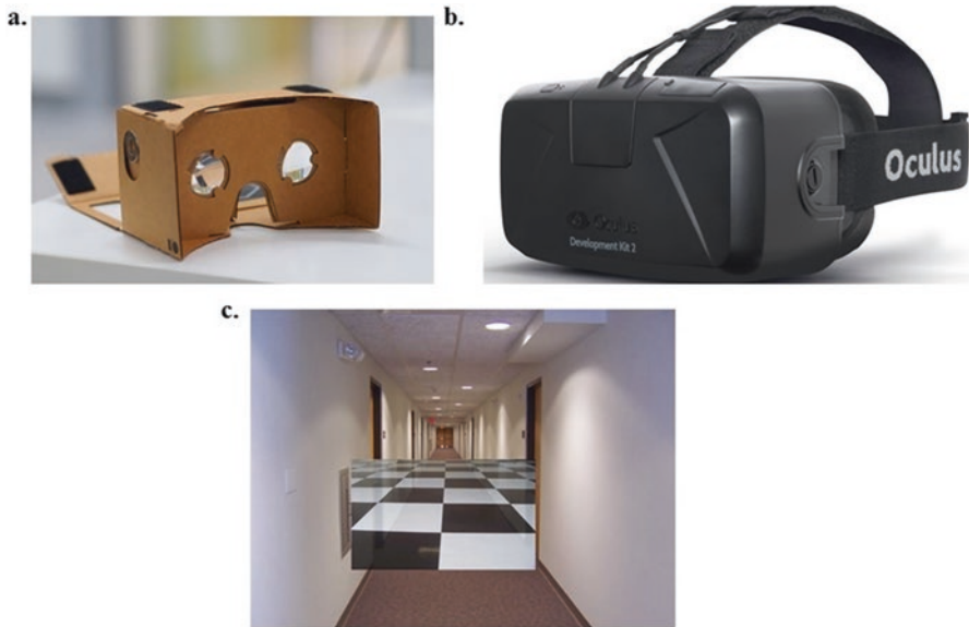
Fig. 10.11 Examples of virtual reality devices and a scenario. (a) The Google™ cardboard goggles provide an affordable alternative to virtual reality glasses using a smart phone, image from Wikimedia commons [78]. (b) Oculus Rift™ virtual reality headset, image from flickr creative commons [79]. (c) An augmented virtual reality scenario for freezing of gait in PD, reproduced with permission from Holmes [80]
