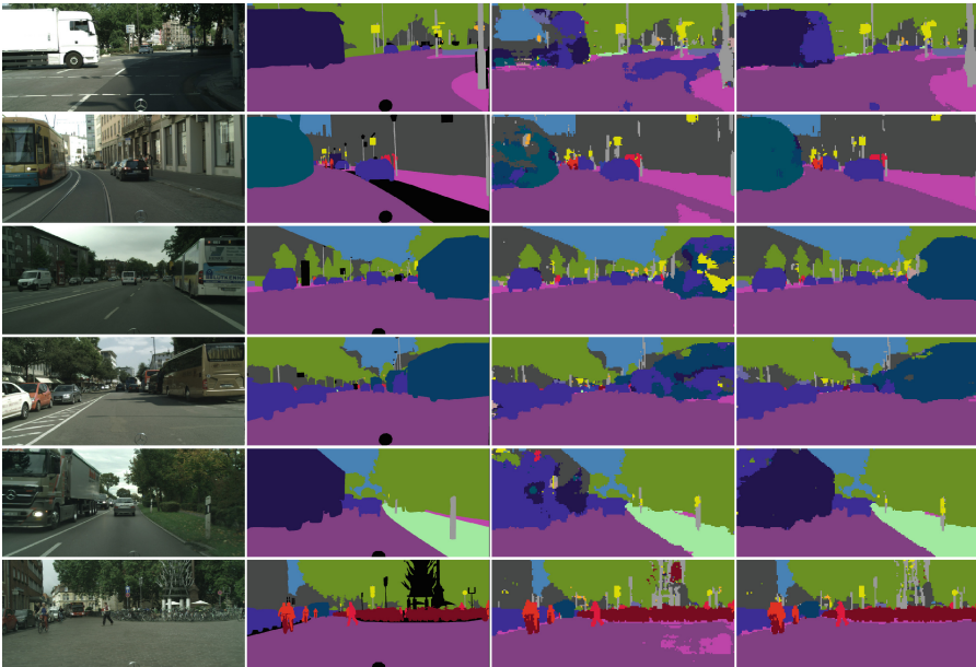
Fig. 4. Examples where scale invariance helps the most. From left to right: input, groundtruth, baseline segmentation (Single3+5), scale invariant segmentation.
