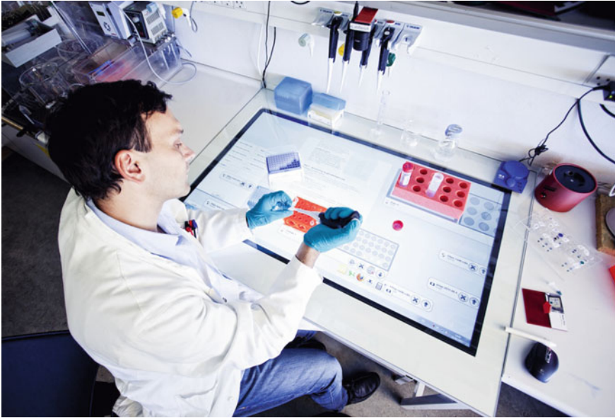
Fig. 11.7 The eLabBench in use by a biologist conducting a lab experiment organized as an activity. Both physical resources, such as the test tube racks, as well as digital resources, such as research articles and a web-based lab notebook, are included in the activity
