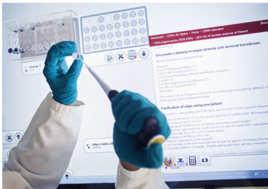
Fig. 11.9 Activity-based Resource Aggregation—When the biologist conducts his experiment, he has access to all relevant resource and these are automatically shown on the eLabBench when resuming an activity. In this case, resources include an annotated testtube rack, the wiki-based lab notebook, and a set of other web sites. The menubar at the lower right allows the biologist to add additional resources to this activity, including websites, a calculator, and a video that records an experiment through the top-mounted camera
