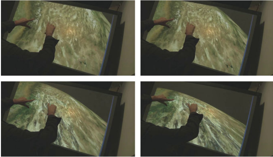
Fig. 6.4 Interaction sequence from the control of the orientation and location of a map orientation in 3D space using 3D-RST [66]. Images courtesy of and © Jason L. Reisman, Philip L. Davidson, and Jefferson Y. Han, used by permission
