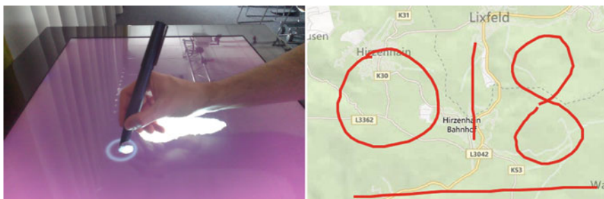
Fig. 14.2 (Left) Touch camera image of pen and hand/arm (after grayscale conversion and filtering); (right) map annotations drawn with an Anoto pen on a Samsung SUR40 tabletop
