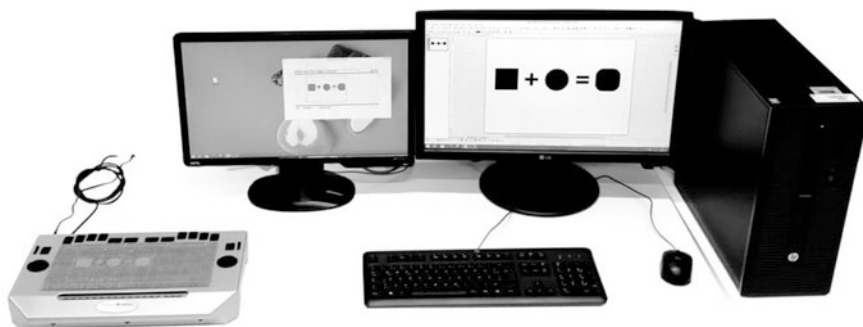
Fig. 19.1 Tangram workstation with the non-visual interface for the blind user (tactile pin-matrix device, left side ) and the visual interface for the sighted user ( right side )
