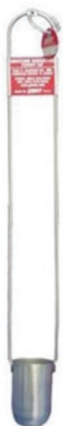
29.13 Photo of Zahn cup (Courtesy of Paul N. Gardner Co., Inc., Pompano Beach, FL) figure
