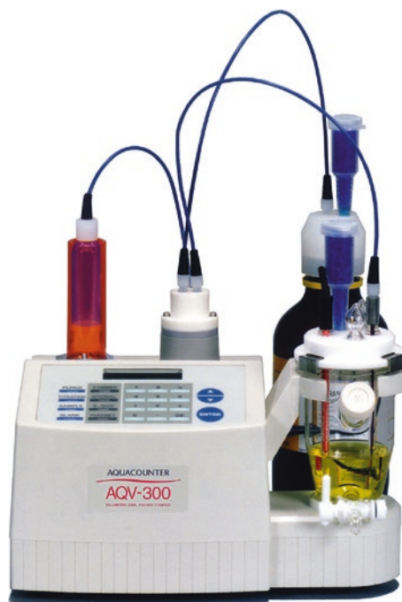
15.5 figure Automated Karl Fischer volumetric titration unit (Courtesy of Mettler Toledo, Columbus, OH)
