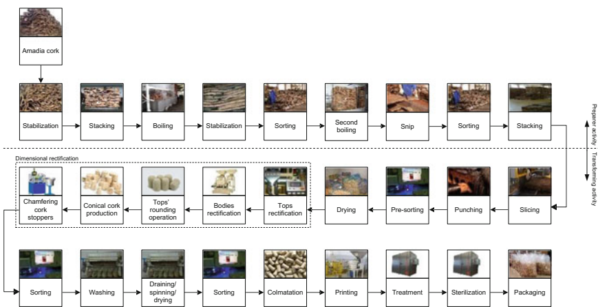
Fig. 1 Natural cork stoppers production industrial processes
