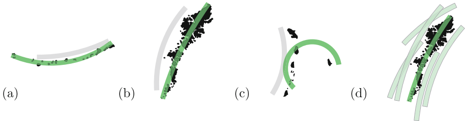
Fig. 9. Island groups with their original, manual label (grey) and the computed label (green). General labels under different points of measurement. (a) Closest point. (b) All points. (c) Closest point. (d) Candidate generation may use general labels to compute several possible high-quality label positions (manual example). (Color figure online)
