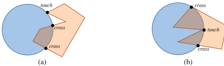
Fig. 4. Two simple scenes with different forms of overlap : (a) a touch-cross-cross sequence, and (b) a cross-touch-cross sequence.
