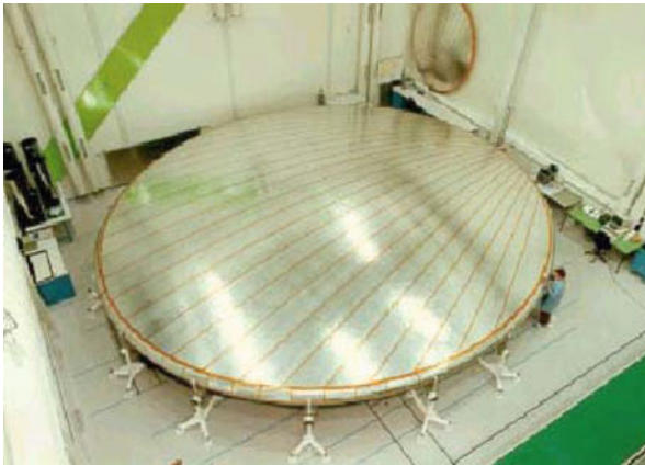
Fig. 4 ESA—Contraves—RUAG (CH) inflatable space rigidized structure (image by Contraves via www.thespaceoption.com/cres_mcbc.php )
