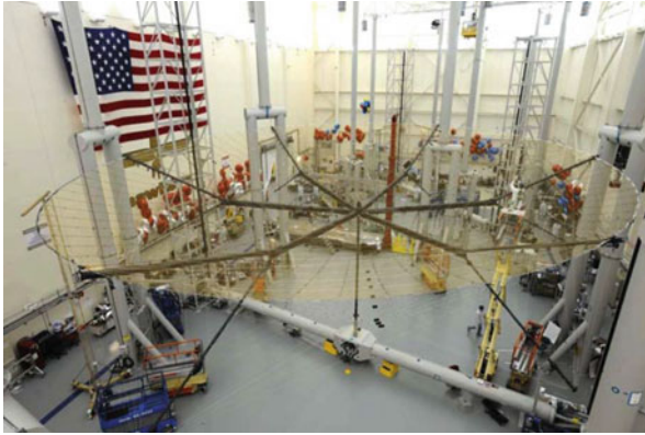
Fig. 2 TerreStar 18 m diameter reflector (image by Harris Corporation, harris.com/harris/whats_new/TerreStar-reflector.jpg )
