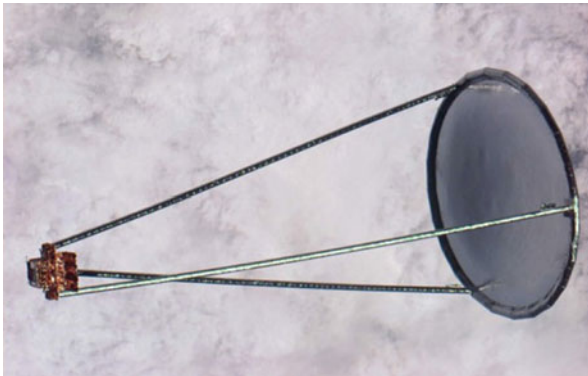
Fig. 5 Inflatable antenna experiment—NASA JPL—L. Garde (image by L.Garde, www.lgarde.com/deployable-antennas.php )
