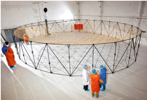
Fig. 1 Astro-Mesh 14 by 11 m peripheral expandable ring concept (image by Northrop Grumman via spacenews.com/northrop-unit-delivers-alphasat-1-xl-reflector/ )
