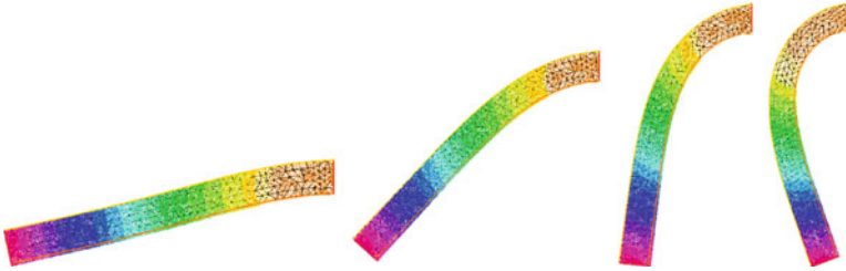
Fig. 2 Free fall under its own weight of the same hyperelastic solid clamped on the left only; position at iteration 50, 100, 150, 200
