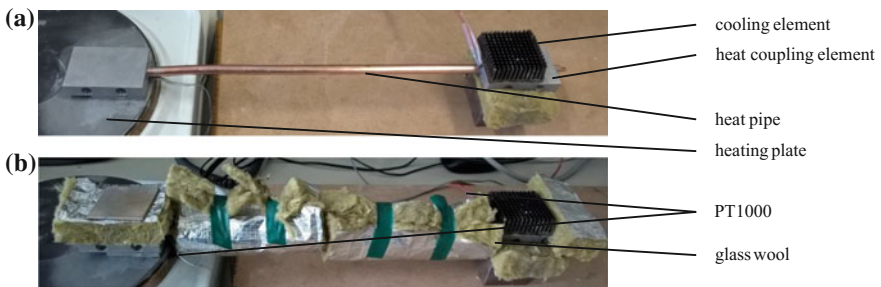
Fig. 2 a Test bed showing the heat source (heating plate), the heat coupling elements on both sides with the heat pipe between them, the cooling element as well as the two temperature sensors (PT1000), b test bed as in a, though completely coated with glass wool
