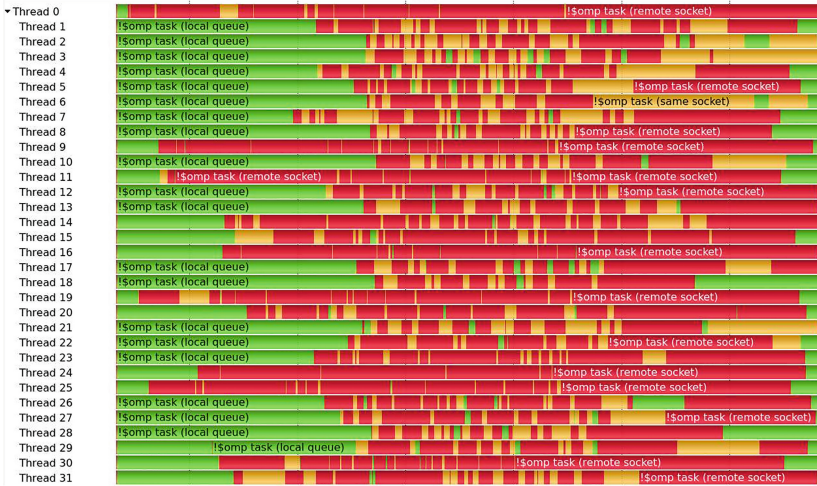
Fig. 6. Vampir screenshot showing the tasks during the execution of the load balancing benchmark with the GNU runtime. Tasks executed on the creating thread are shown in green, stolen tasks from the same NUMA-node in orange and from remote NUMA-nodes in red. Comparing this figure to Fig. 5, a huge difference in the way tasks are scheduled in the GNU and Intel runtime can be observed. (Color figure online)
