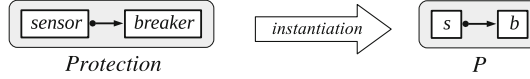
Fig. 2. Active-system model Protection (left) and its instantiation into active system P (right)
