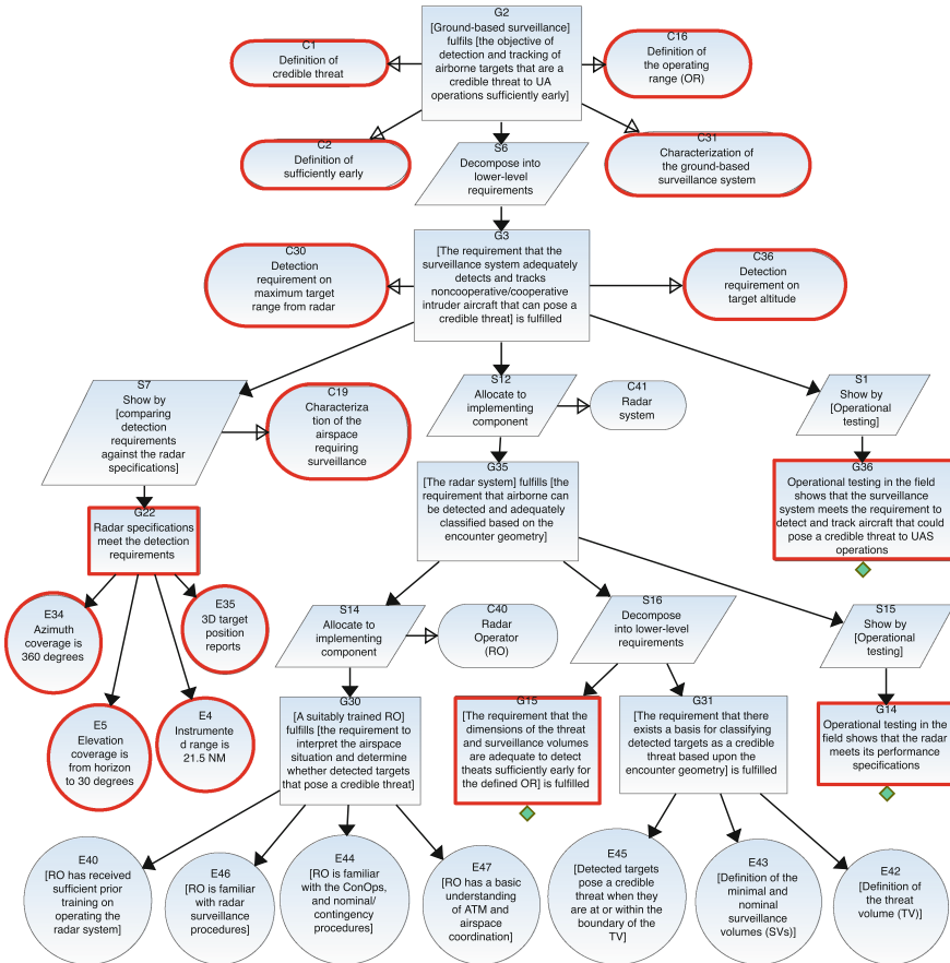
Fig. 3. Fragment of the instance argument of the compound pattern in Fig. 2, when instantiated for the surveillance barrier, and appended with tailored argument elements (shown by the goal, context, and solution nodes highlighted with a thick border).
