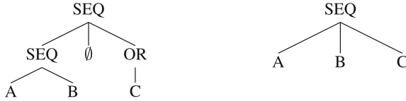
Fig. 3. Two process trees modeling exactly the same behaviour. The left model is reducible, and the right model is its irreducible representation. The silent transition \emptyset is removed because it is not part of an OR structure. The OR elementary node does not provide behavioural information.
