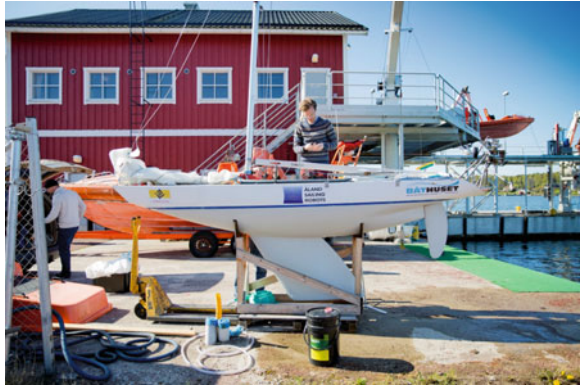
Fig. 1 Åland Sailing Robots Mini 12 sailboat, which shall be fitted with a wingsail
