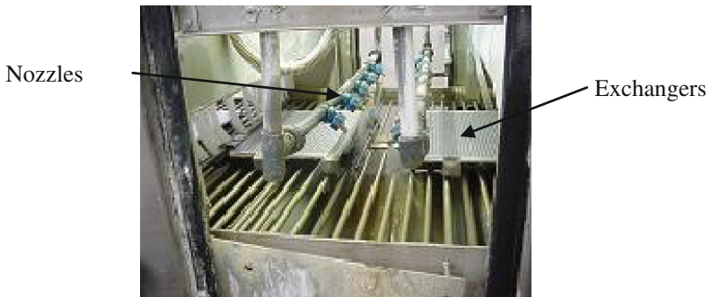
Fig. 9. Spraying process to apply flux on external surfaces of exchangers
