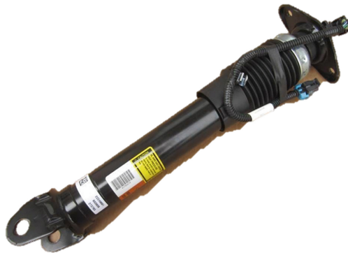
Fig. 3. The tested magneto-rheological shock absorber (Chevrolet Corvette)
