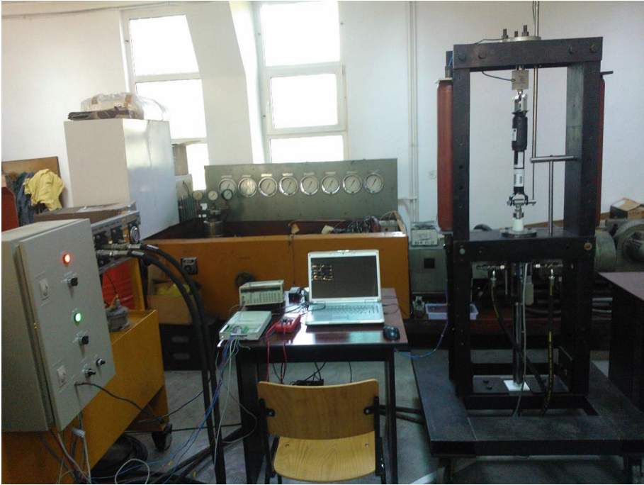
Fig. 4. Partial view of the magneto-rheological shock absorbers test bench
