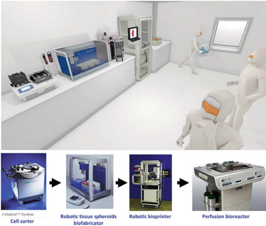
Fig. 4 Organ biofabrication line (scheme)
