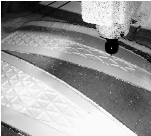
Fig. 8 Petal fabrication on CNC milling-machine
