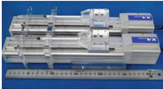
Fig. 5 External appearance of syringe used to feed and aspirate driving fluid in the main body of the catheter and linear slider used for reciprocating motion of syringe piston (323.5 mm long by 111.0 mm wide)
