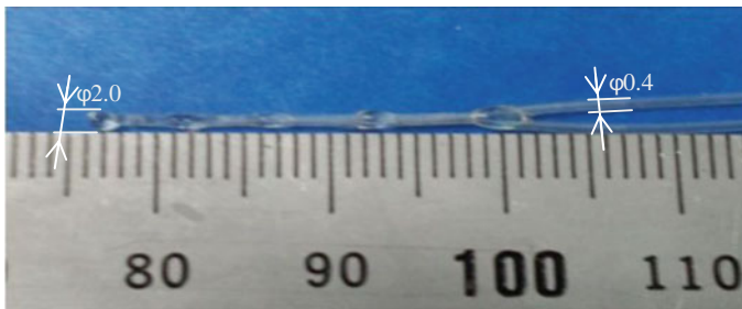
Fig. 3 External appearance of catheter developed in our laboratory [23.0 mm long by \phi 2.0 (feeding pipe \phi 0.4)]
