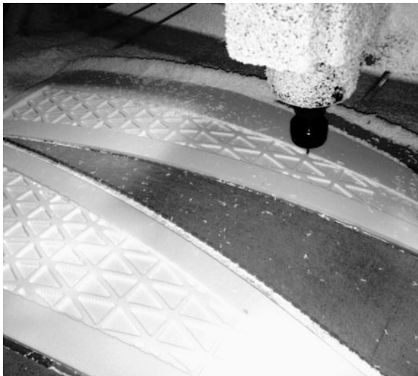
Fig. 8 Petal fabrication on CNC milling-machine
