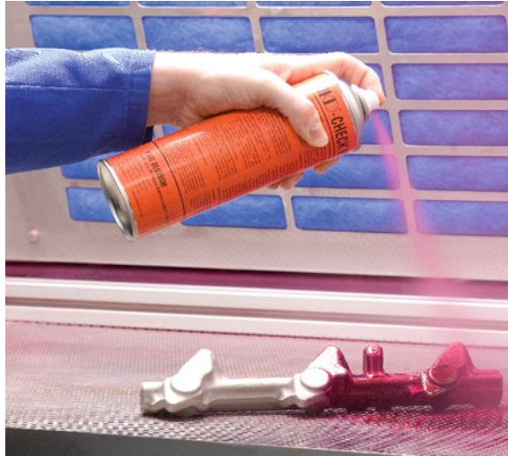
Fig. 1 Inspection employing penetrating liquid
