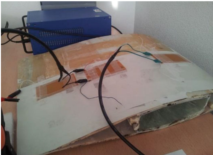
Fig. 3 Installation of sensors on a blade in the laboratory
