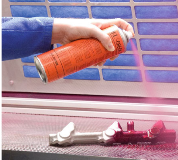
Fig. 1 Inspection employing penetrating liquid
