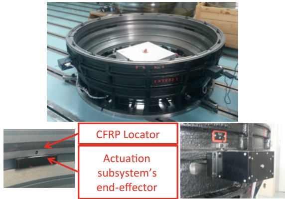
Fig. 2.10 Fixture assembly and detail of the actuation subsystem assembly ( Left External view; Right Internal view)
