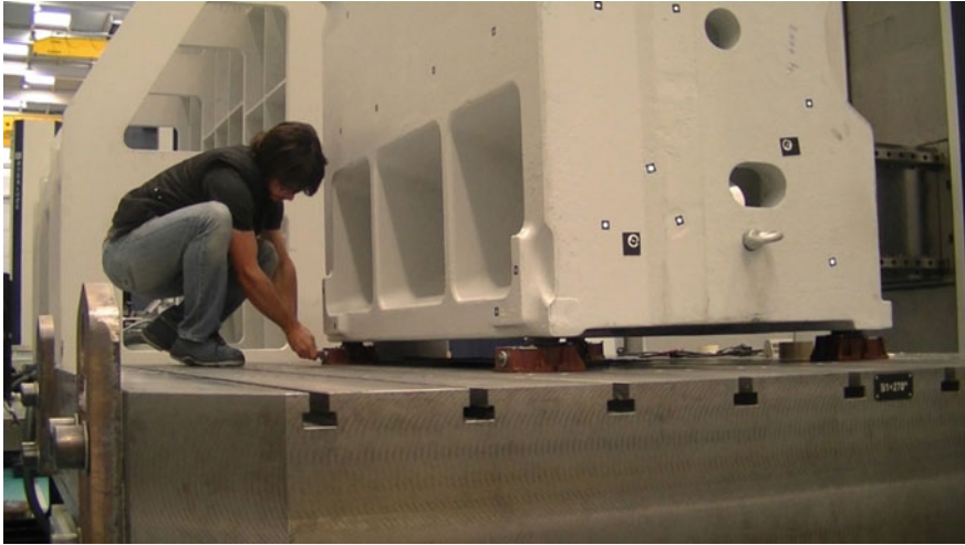
Fig. 9.2 Manual alignment of a workpiece in a milling machine
