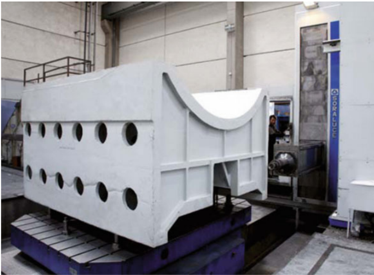
Fig. 9.1 Large prismatic part in a milling machine
