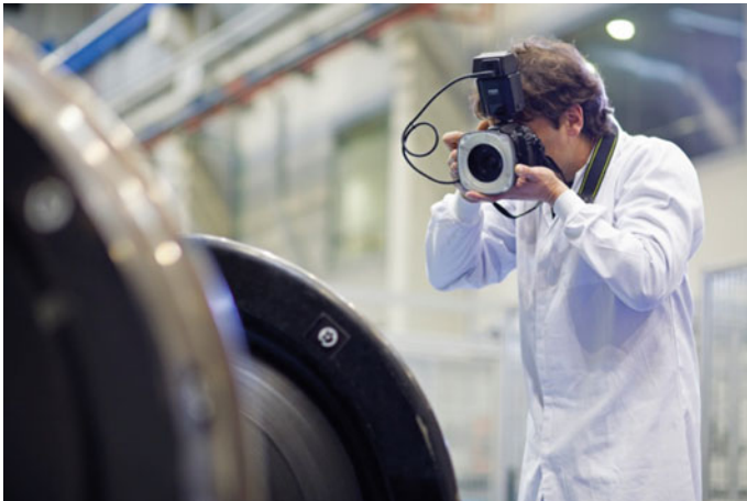
Fig. 9.6 Out-of-machine photogrammetry setup
