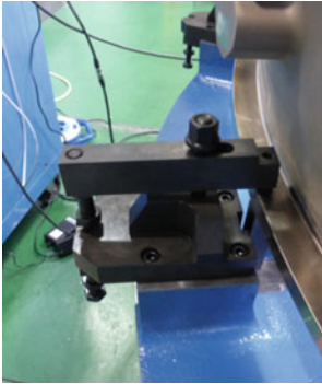
Fig. 7.3 Detail of an axial clamping element and clamping area of the workpiece
