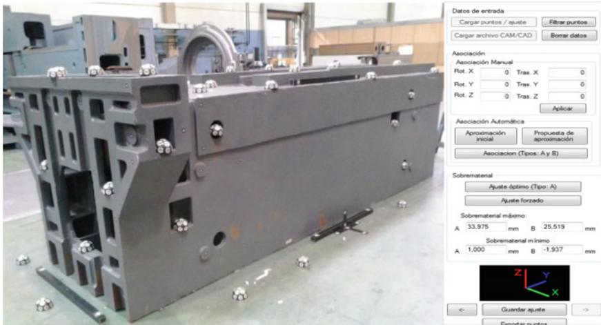
Fig. 9.16 Validation of system with grinding machine column: characterization ( left ), screenshot of application ( right )
