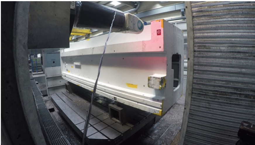
Fig. 9.17 Raw part located on the machine table with markers
