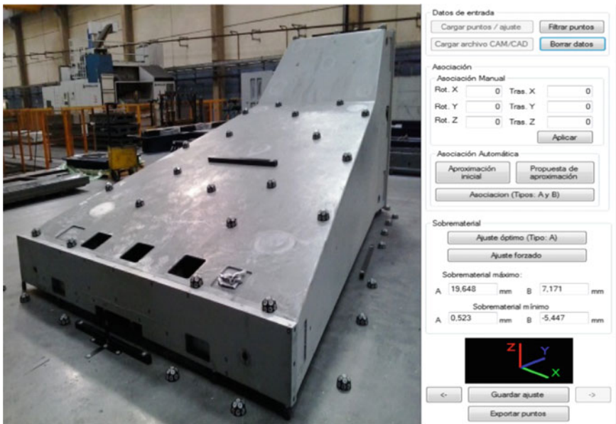
Fig. 9.15 Validation of system with gantry type machine column: characterization (left), screenshot of application for adjustment and calculation (right)
