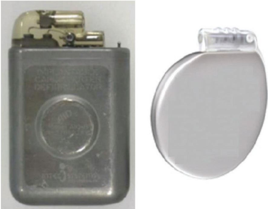
Fig. 13.1 Original implantable cardioverter defibrillator pulse generator, on the left , and a modern device on the right (Gasparini and Nisam [17]. [16] Copyright 2016 by Springer)
