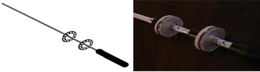
Fig. 2 A prototype of an ablation probe with two LED rings
