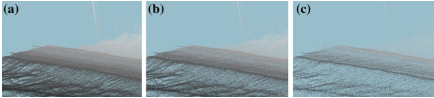
Fig. 6 Results of the random tree sampling. The point cloud in a with the highest density shall be loaded for the nearest node, while b is less dense and will be loaded for the middle-distanced node. The least dense c will be loaded for the far-away nodes. Farthest nodes will not show any points
