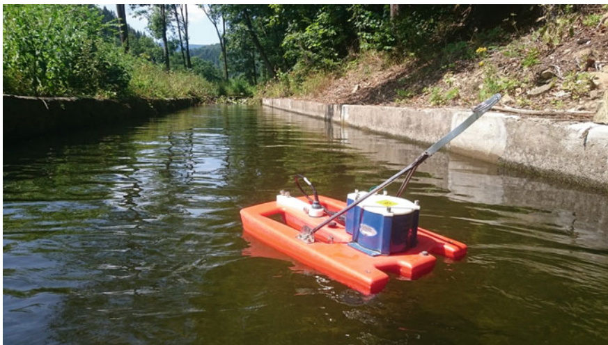
Fig. 7 ADCP RDI StreamPro during measurement in Hanušovice flume
