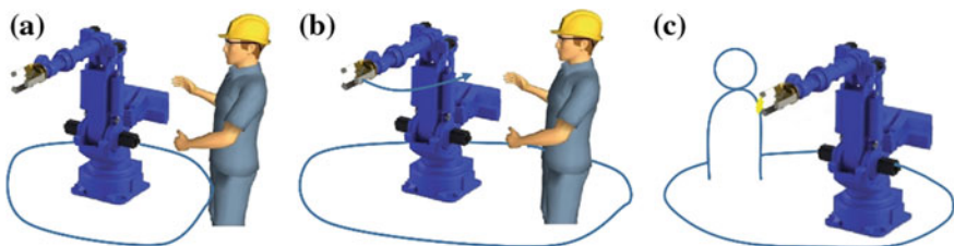
Fig. 4.2 Collaboration classification. a Robot on safe hold against human violation. b Speed reduction even the worker is in the robot work zone. c Robot touching the human with a pre-defined calibrated force
