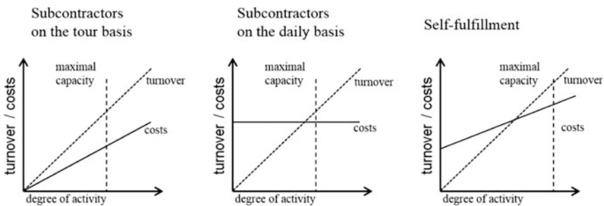
Fig. 24.1 Comparison of costs for different types of subcontraction and self-fulfillment (cf. Kopfer and Krajewska 2007)
