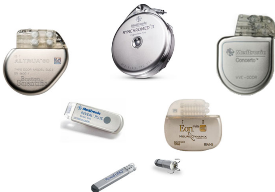
Fig. 18.7 Implantable electronic devices. Top row: pacemaker, drug pump, defibrillator. Second row: pressure monitor, neurostimulator. Third row: loop recorder, transcatheter pacemaker
