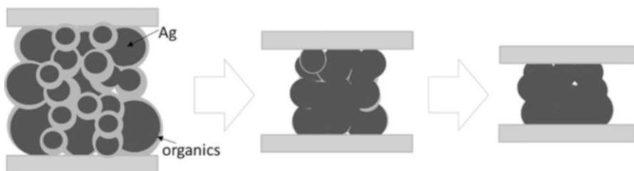
Fig. 14.4 The schematic diagram of sintering process for hybrid Ag paste
