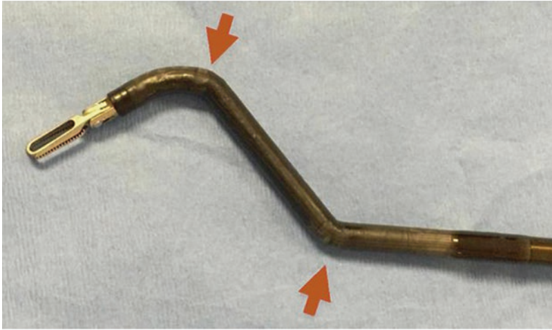
Fig. 33.6 EndoWrist forceps showing the double-jointed distal end with elbow and articulating wrist joints that facilitate triangulation at the surgical site
