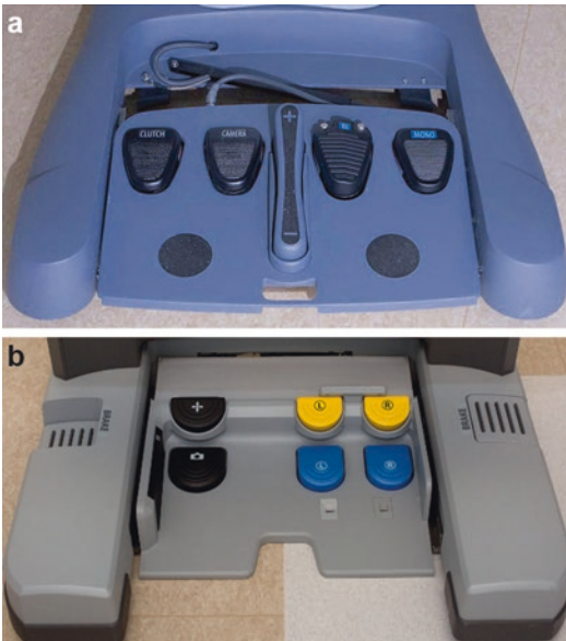
Fig. 3.10 Photograph of foot switch panels from the da Vinci® S (a) and Xi (b) systems with pedals for clutch, camera, focus control, accessory/bipolar, and monopolar electrocautery
