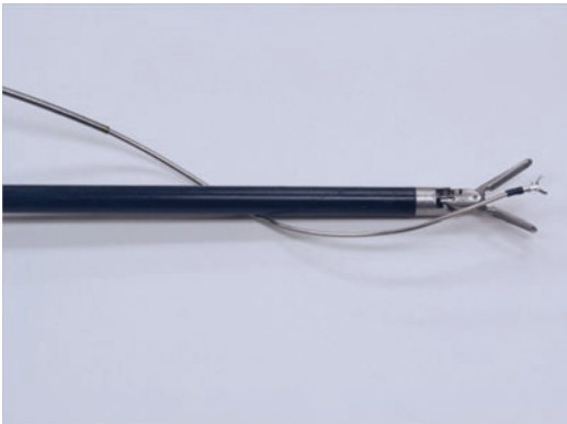
Fig. 34.5 Concentric tube robot with microlaparoscopic sized end-effector manipulator (grasper) compared to standard da Vinci instrument
