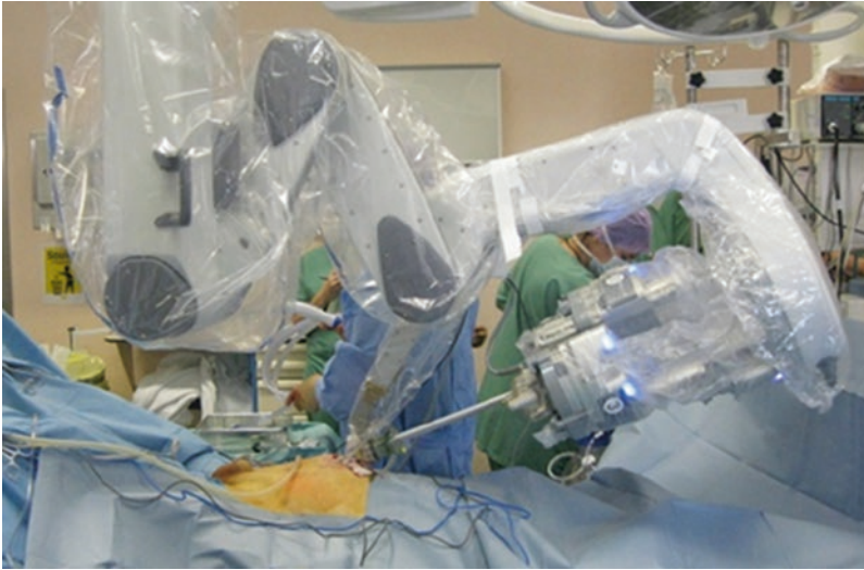
Fig. 33.5 Docking of SP999 robotic system
