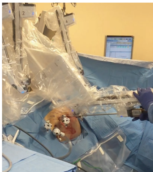
Fig. 11.4 With the Da Vinci S and Si, a 12 mm camera port was required. However, with the Da Vinci Xi any of the 8 mm ports can be used
