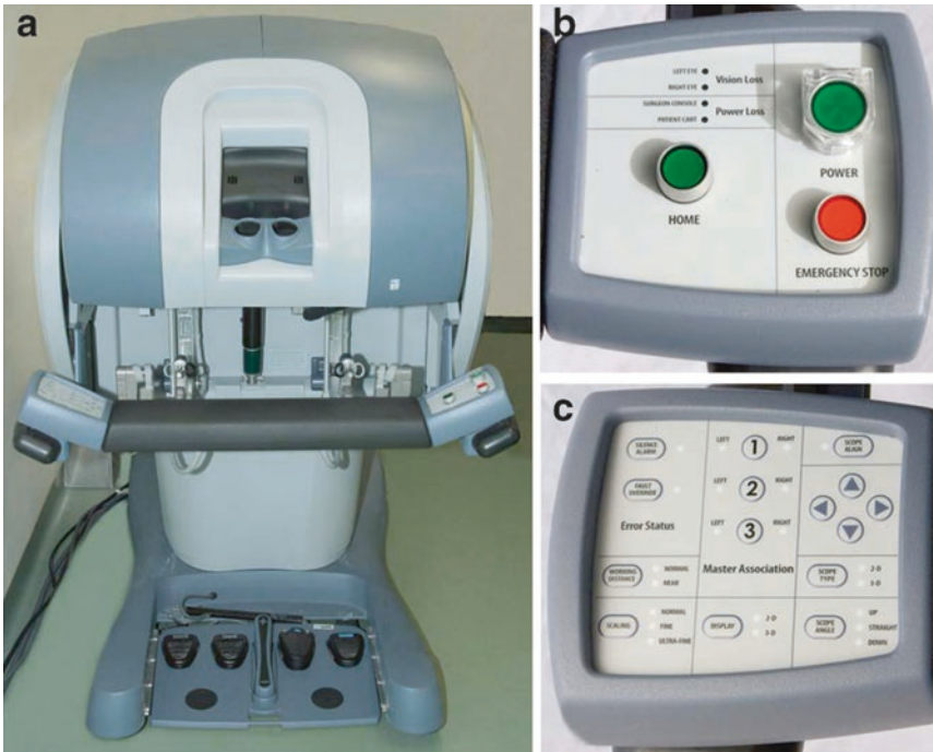
Fig. 3.6 Photograph of da Vinci® S surgeon console (a), right (b), and left-side (c) pod controls
