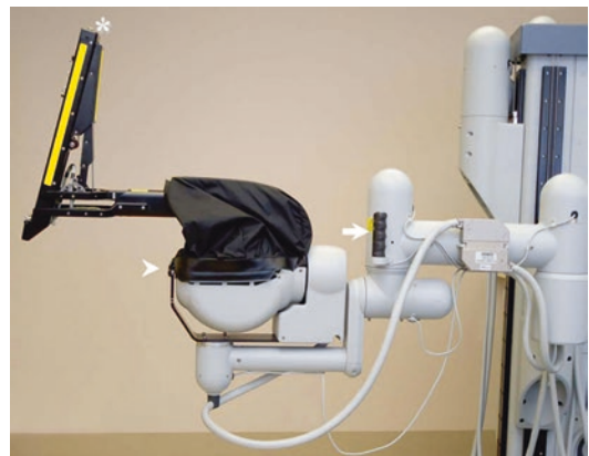
Fig. 3.12 Photograph of the da Vinci® standard instrument arm showing the port clutch joystick button ( arrow ), port clutch button ( arrowhead ), and instrument clutch but-
