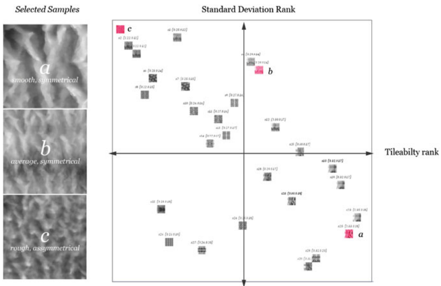
Fig. 10 Operation 3, sorting. Interactive graphs plot texture samples generated by the design tool with respect to design criteria such as variation and tileability
