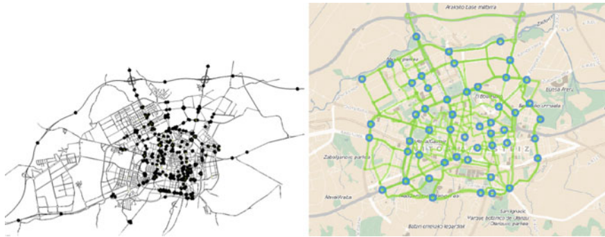
Fig. 11.3 The Vitoria network, Basque Country, Spain: Loop detector sensors layout ( left ) and AVI Bluetooth detectors layout ( right )
