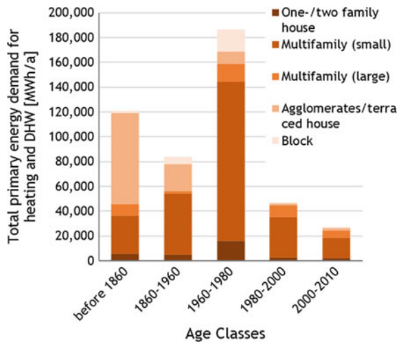
Fig. 3 Primary energy demand for heating by building typologies and age classes before renovation
